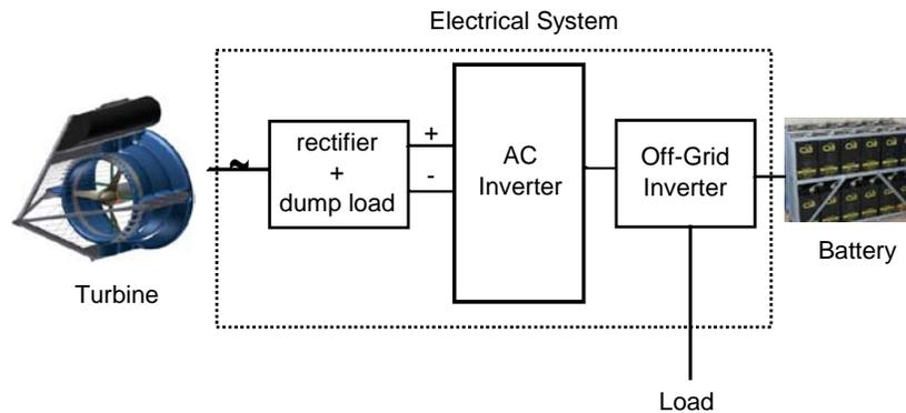
**Fig. 10: Electrical System connected the output of the turbine**
