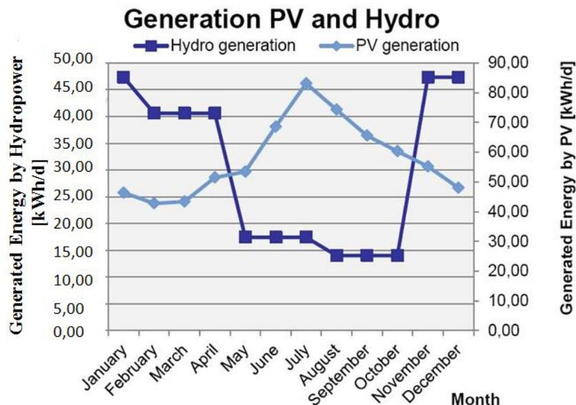
**Fig. 14: Yearly generation through a Hydrokinetic and Photovoltaic hybrid system**
