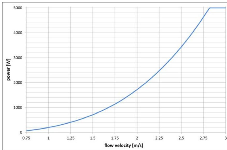
**Fig. 11: Operating curve of SMART Monofloat Kinetic Micro Hydro Generator**
