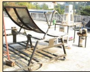
Solar Energy based efficient plant for preparing Turpentine oil and Rosin from Pin Resin
