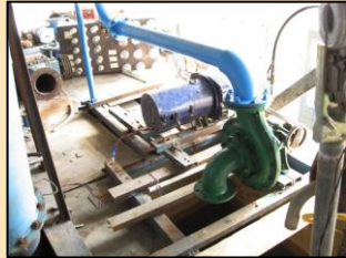
Modified Pump used as Turbine
